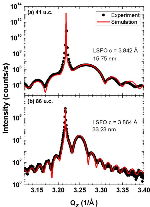
FIG. 1. X-ray diffraction and simulations of (a) 41 u.c. and (b) 86 u.c. of LSF0 on (001) STO.
