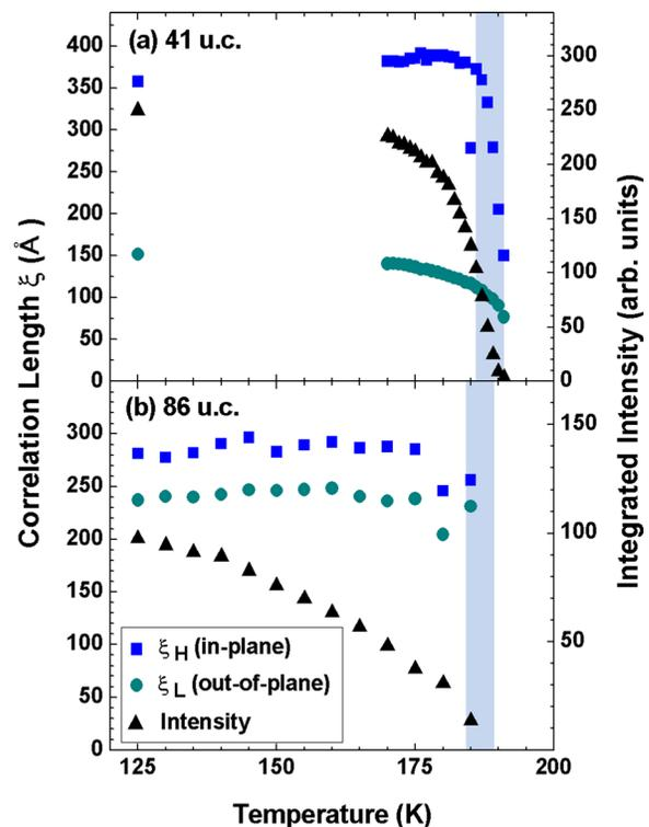
FIG. 4. Correlation lengths and integrated intensity of the  $(4/3\ 4/3\ 4/3)$  reflection from the (a) 41 u.c. and (b) 86 u.c. films.
