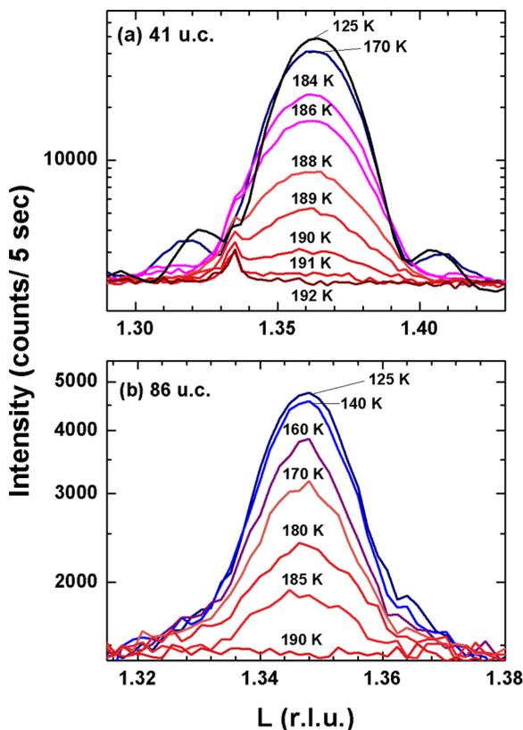
FIG. 3. The  $(4/3\ 4/3\ 4/3)$  reflection from (a) 41 u.c. and (b) 86 u.c. films. Above the transition temperature,  $T^*$ , no reflection is observed. The small, sharper peak in (a) at  $L = 1.335$  comes from a higher harmonic x-ray diffracting from the substrate. The reciprocal lattice units are given with respect to the  $\text{SrTiO}_3$  substrate.
