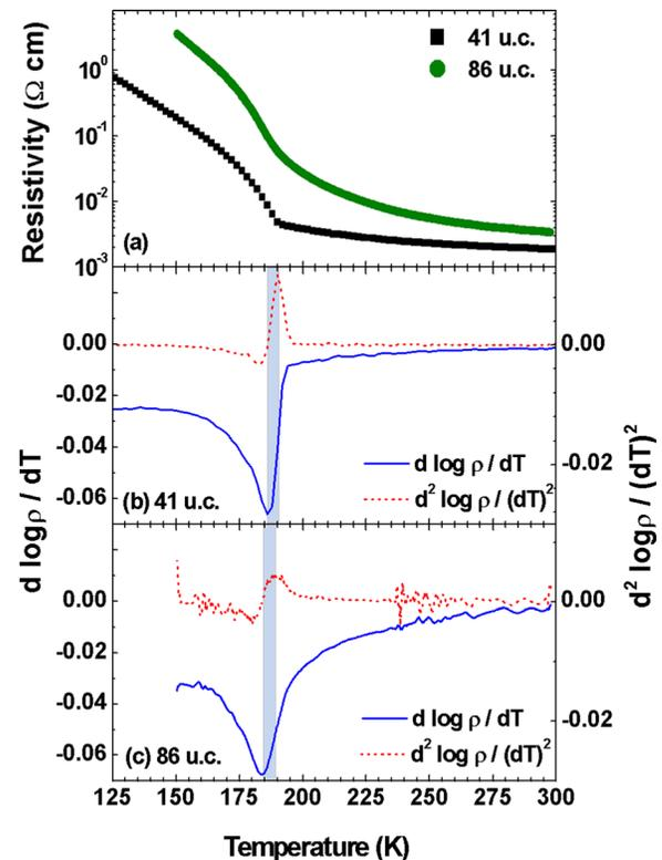
FIG. 2. Resistivity as a function of temperature for the two LSF0 films (a); derivatives of resistivity with respect to temperature (b) and (c).
