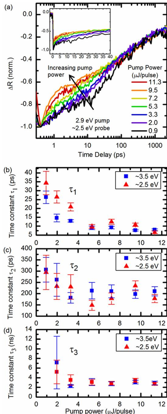
FIG. 4. (a) Normalized kinetic traces and (b)–(d) fitted time constants as a function of pump power. The pump energy is 2.9 eV and probe energies are indicated in each panel.
