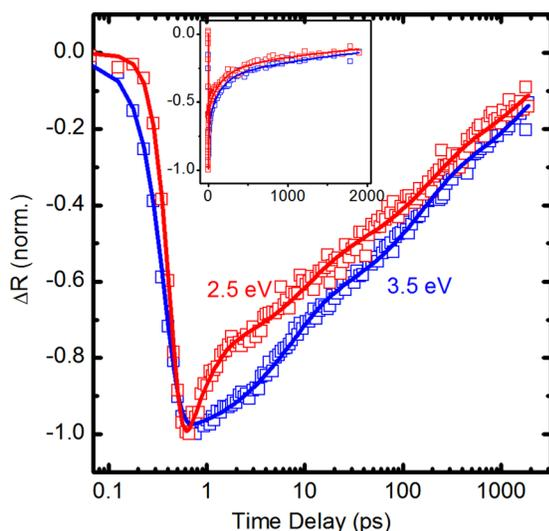
FIG. 3. TR kinetics for probe energies of  $\sim 3.5$  eV and  $\sim 2.5$  eV, with log and linear (inset) time axes, after photoexcitation at 4.0 eV with 6.9  $\mu\text{J}/\text{pulse}$ . Symbols are experimental data and lines are the fitted model.
