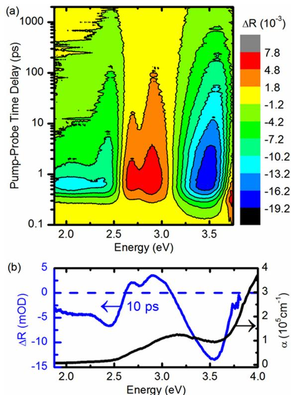
FIG. 2. (a) 2-D contour plot showing  $\Delta R$  as a function of probe energy and pump-probe delay time. The pump energy was 4.0 eV at a power of 6.9  $\mu\text{J}/\text{pulse}$ . (b) A 1-D slice from the contour plot showing  $\Delta R$  versus probe energy at a delay time of 10 ps, along with the absorption coefficient obtained from spectroscopic ellipsometry.
