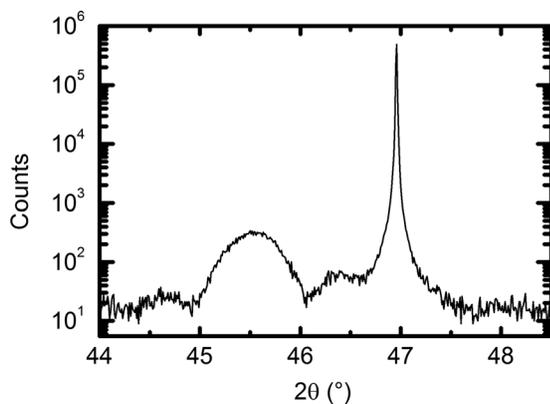
FIG. 1. X-ray diffraction obtained from the (002) peak of the LFO film on a LSAT substrate.
